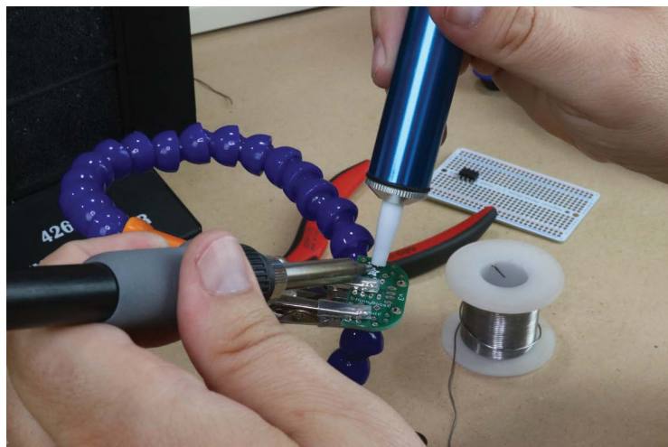
FIGURE 4-10: Component that needs the solder removed with a solder sucker
