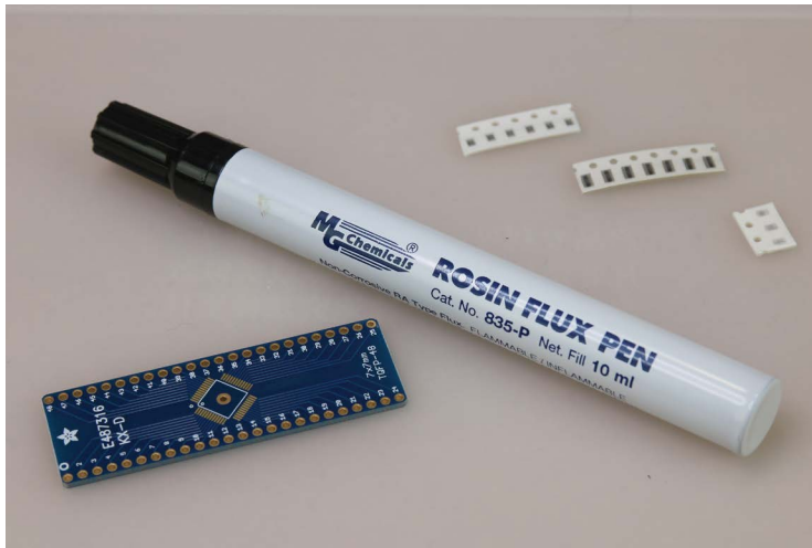
FIGURE 5-10: A flux pen is a must when surface-mount soldering.
