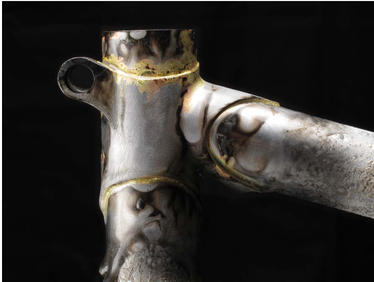
FIGURE 1-6: Brazed seat lug from "Building a frame" by Phil Gradwell IMAGE COURTESY OF FLICKER COMMONS, LICENSED UNDER CC BY 2.00
