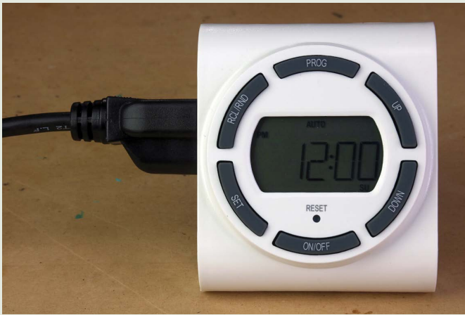
FIGURE 2-15: Soldering iron plugged into a standard electrical timer
